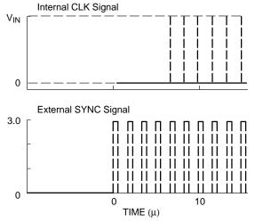
Figure 3. Timing Diagram of the SYNC Signal
