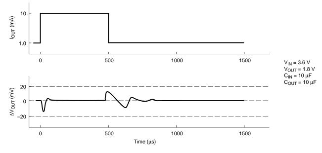
Figure 5. Load Transient Response in Linear Mode
