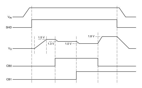
Figure 7. Power–Up and Power–Down Sequence
